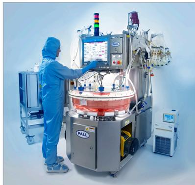
1 x 333 m<sup>2</sup> iCELLis 500+ Bioreactor
