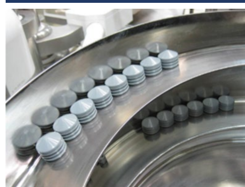
Figure 7: Plungers moving well orientated up the Vibratory Sorting Bowl - the image is property of Syntegon
